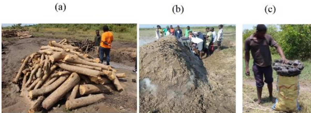
Figure 5.2. Mangrove wood usage for charcoal production: (a) woods of Xilocarpus granatum piled up for charcoal stove, (b) a charcoal stove burning and (c) a bag of charcoal produced. (Bairro Aeroporto, Chinde, Zambezi Delta, October 2016).
